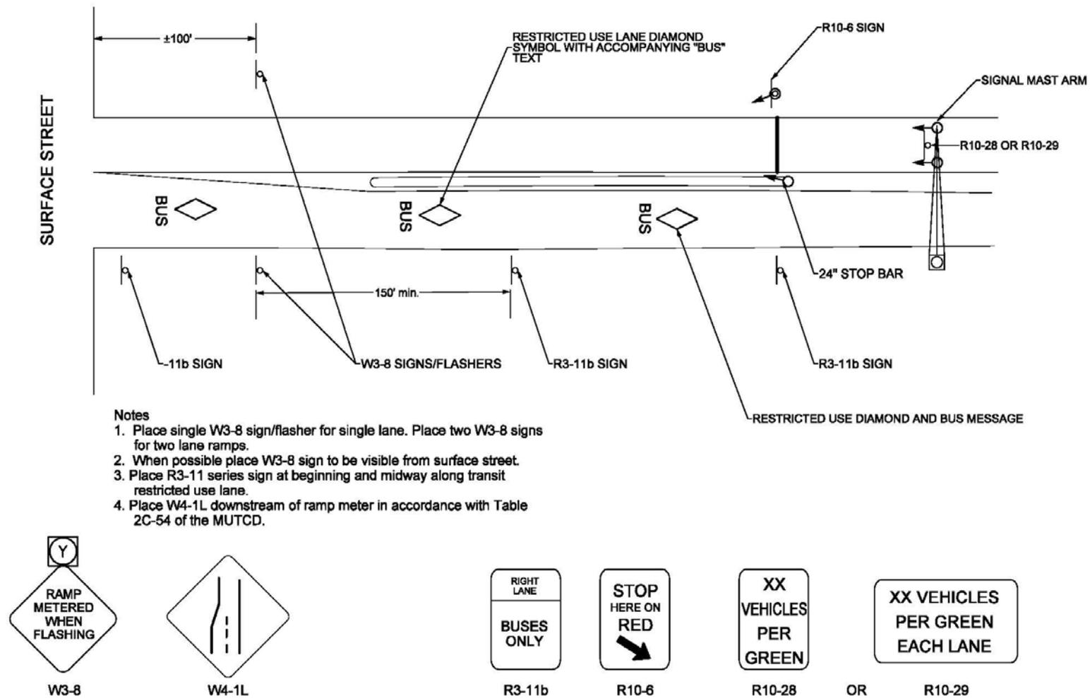
Figure E-1: Non-Freeway-to-Freeway Ramp Meter Signing and Pavement Markings
