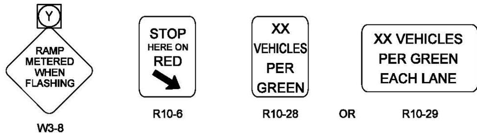
**Figure E-2: Single-Lane Loop Ramp Meter Signing and Pavement Markings**
