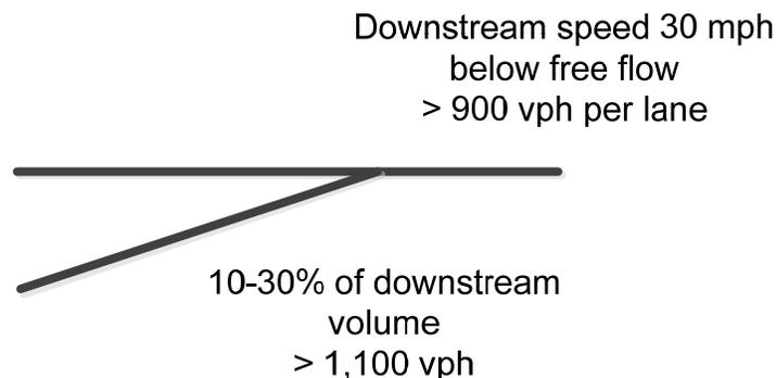
**Figure 1: Typical Criteria for Ramp Metering**
